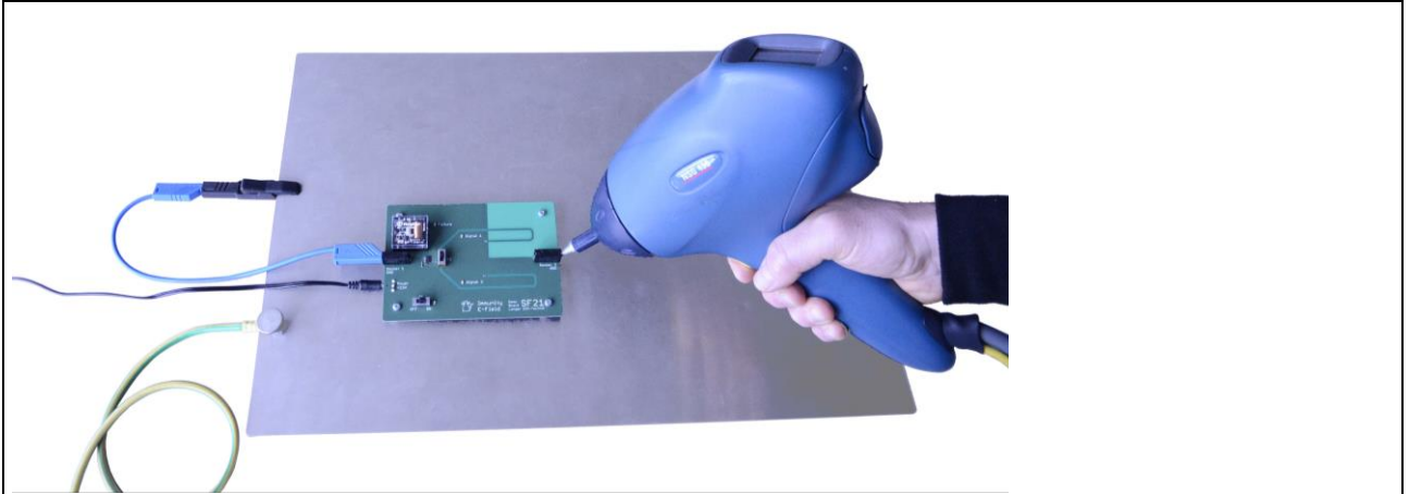
Figure 23: Experiments with ESD generator over a metal surface
